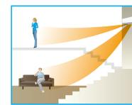
Mitsubishi Electric's double vane separates the airflow in the left and right directions to deliver airflow not only across a wide area of the room, but also simultaneously to two people in different locations.
